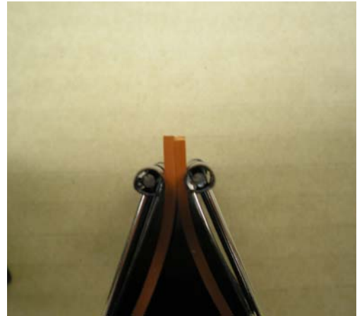
Photo II – Benchmark Material After 24 hr @ 300°C
