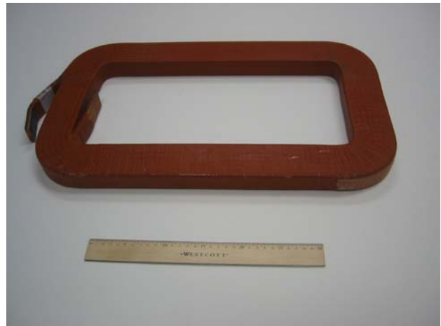
Figure 1 -Main field coil from a DC traction motor wrapped with silicone Traction Motor Tape.
