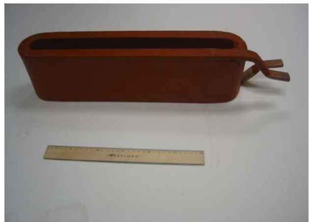
Figure 2 - Interpole coil from a CD traction motor wrapped with silicone TMT
